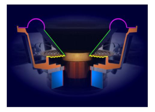
As soon as current from the amplifier flows in the voice-coil it produces a magnetic field that interacts with that of the magnet. This forces the voice-coil to move, together with the cone with which it is integral. The shift and direction of this moving element are determined by the intensity and direction of the flow in the coil.
