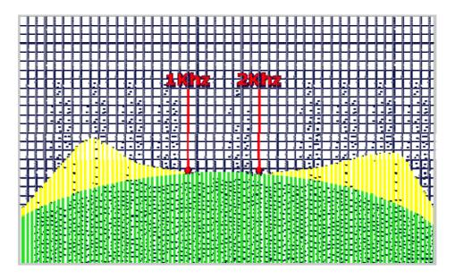
Both to resonance of the midrange and to the highest frequencies, the filter sees a greater load impedance and filters less. Result: the curves are equal only in the octave 1Khz–2Khz while the portions of frequency that the filter had to reject are instead in overbearing evidence. Really awful!
