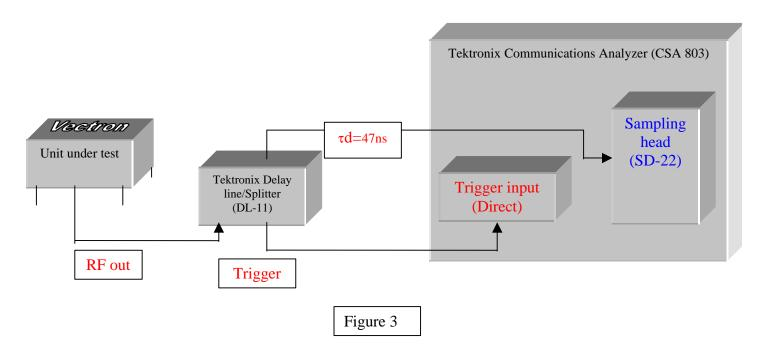
The output of the unit under test is fed into splitter /delay line. The non-delayed output of the splitter is fed to the external trigger input of the oscilloscope (a CSA-803 in this case). The delayed output of the DL-11 is connected to the input of the oscilloscope. By
