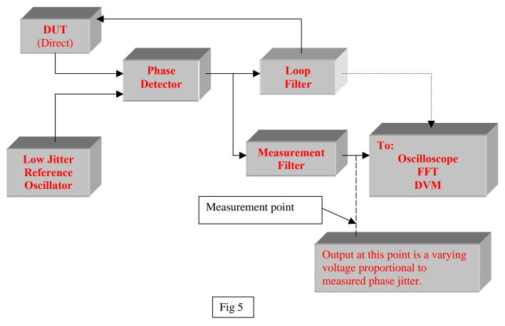
Figure 4 shows the basic elements of a phase locked loop (PLL) used to measure the noise of a clock source. Gardner [5], Best [6], and Woolover [7] are three excellent references for understanding PLLs. Some key loop requirements follow:
