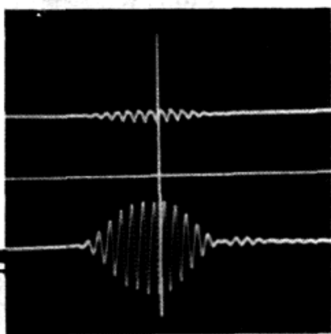
Fig. 19 — Response to 10.8-kHz tone burst from Shure TTR-103 test record, band 4, 30 cm/S peak at 45 degrees. The echo appears to be an artifact of the record.
